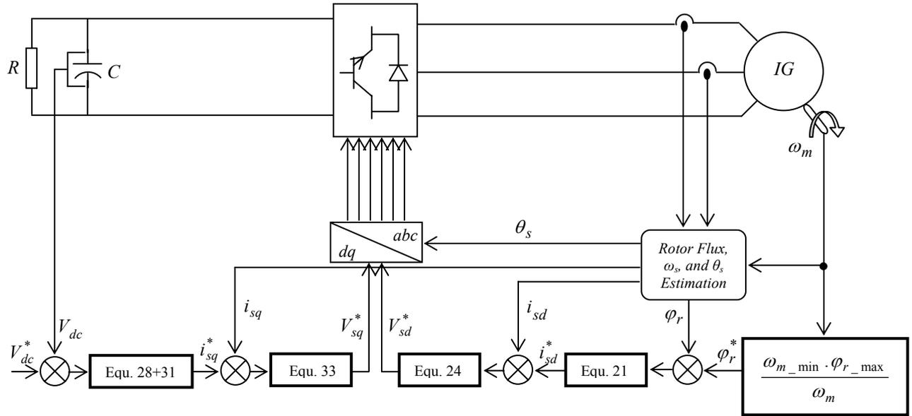
Fig. 1. Control structure proposed
