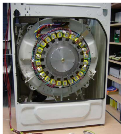
Fig. 1: Prototype of a Flat shaped Switched Reluctance Motor fitted to a tub of a washing machine.
