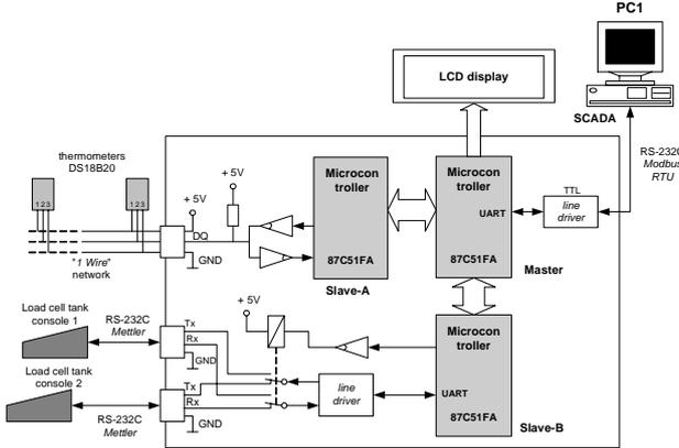
Fig. 3. Functional diagram of the hardware unit developed to integrate load cell tank consoles and a network of digital thermometers.
