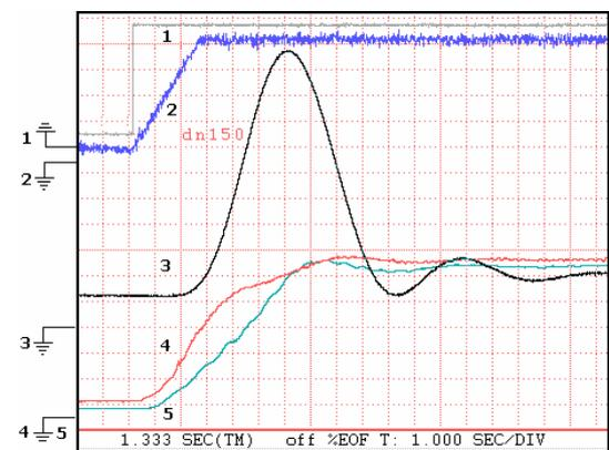
Fig. 9. Flow-rate response (3) to a ramp speed pump variation (2); Speed signal imposed to the variable speed pump drive (1); Pressure sensor in the centrifugal pump (4) and in the flow-meter pipe column (5); Motor group 2 and 150 mm diameter pipe.
