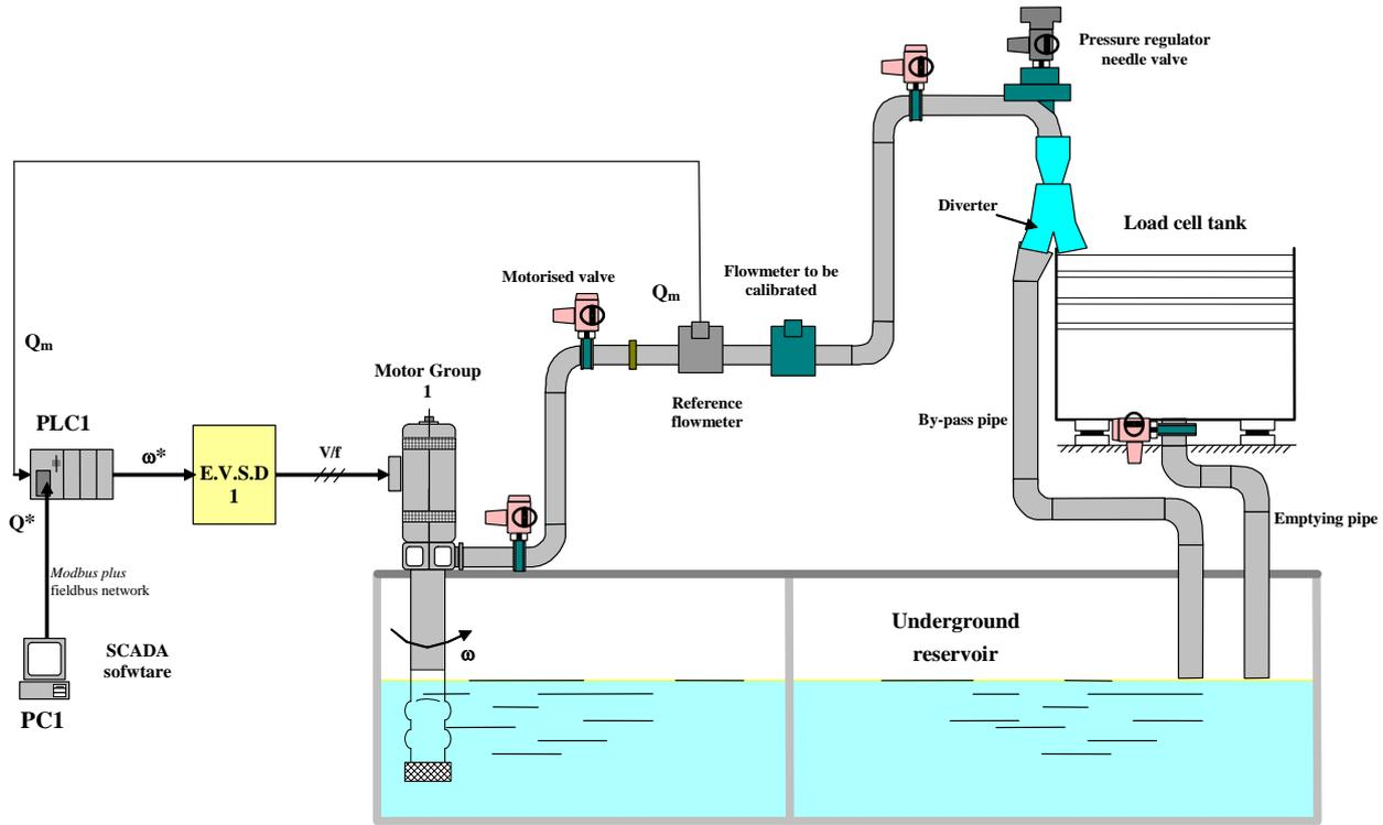
Fig. 10. Block diagram and synoptic description of closed-loop flow control devised for the flow-meter calibration section.
