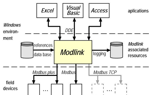
Fig. 13. Modlink software connections.
