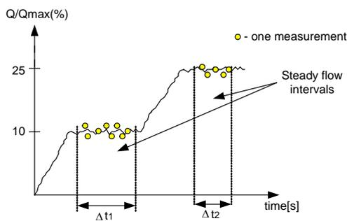
Fig. 7. Typical measurement steps at constant flow-rates.
