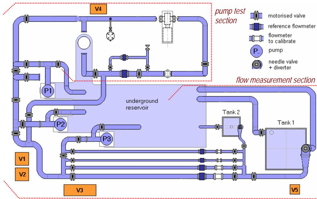
Fig. 1. Simplified plant view showing schematically the hydromechanical equipment of LEHid.
