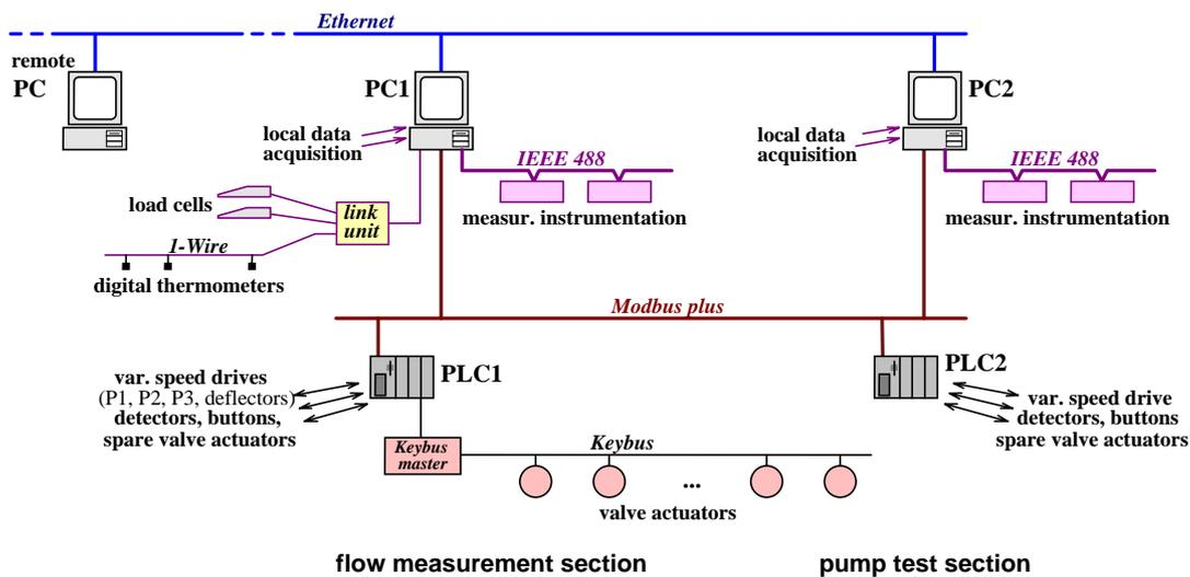
Fig. 2. Automation structure at LEHid.
