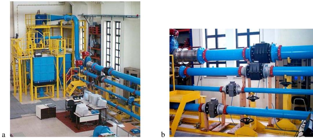
Fig. 6. a) Downstream view of flow measurement section; b) view of the set of reference electromagnetic flow-meters.
