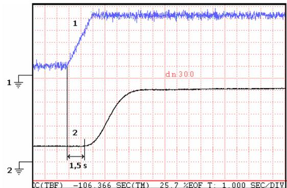
Fig. 8. Flow-rate response (2) to a ramp speed pump variation (1); Motor group 1 and 300 mm diameter pipe.
