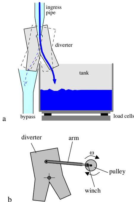
Fig. 4. Bi-directional motion of a diverter: a) tank filling process; b) pulley-arm transmission system.
