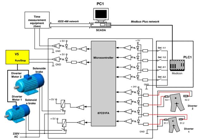
Fig. 5. Functional diagram of the hardware unit developed to control motion of the diverters.
