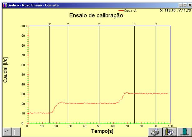
Fig. 11. Sample diagram of the flow-rate transient response in closed-loop control (steps of a calibration procedure).
