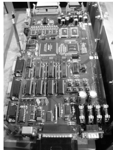
Fig. 6. Photography of the control board based on the TMS320LF2407 DSP
