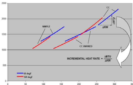
Figure 7. HR thermal consumption c. cycles functions.
