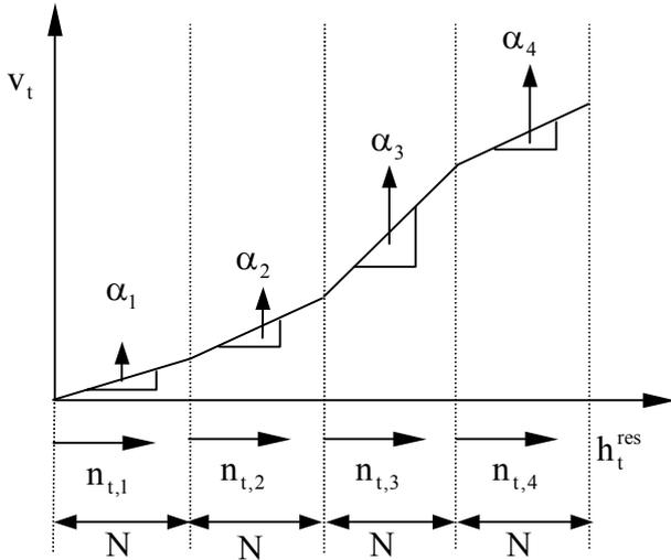
Figure 3. Piece-wise approximation of the relationship between the reservoir volume and its height. Four blocks are used.
