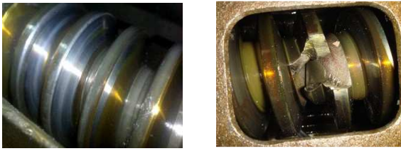
Fig. 2: Detail of a worm showing surface wear (left); detail of a broken worm (right).
