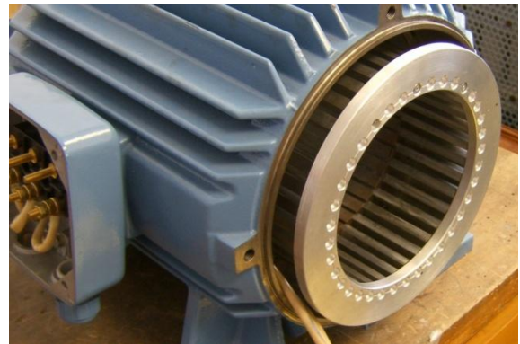
Fig. 3– Stator of the inverted induction motor.
