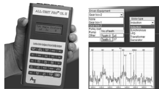
Figure 2. Industrial Equipment to detect failures in motors.
