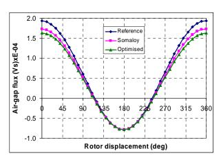
Fig. 6. Air-gap flux characteristics
