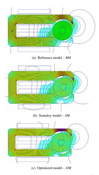
Fig. 4. Magnetic flux plot at peak–torque regime  $\delta_{max}$ =90°
