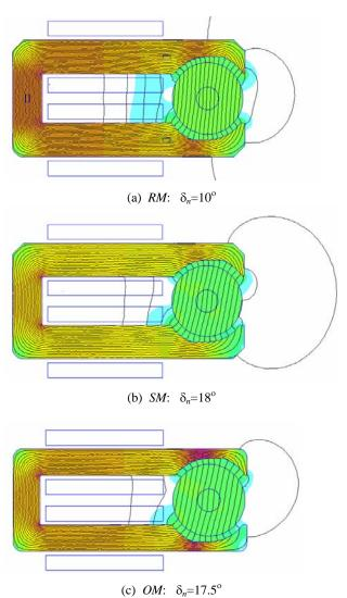
Fig. 3. Magnetic flux distribution at rated current  $I_n$ =0.25A
