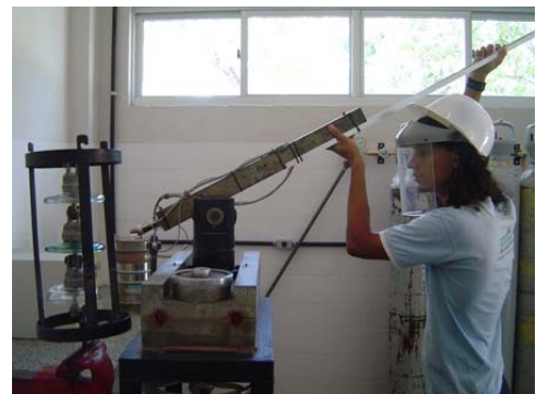
Fig. 8. Fixing of the hose and rotating mechanism
