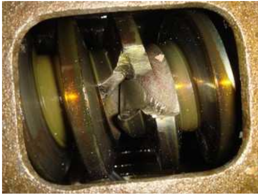
Fig. 4: Detail of a broken worm.
