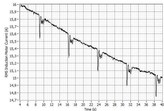
Fig. 7: The induction motor current was measured at 310 RPM.
