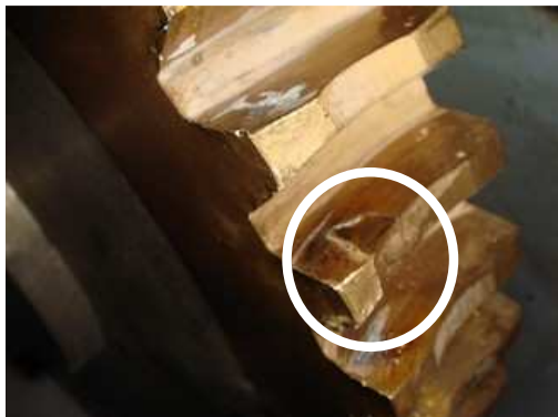
Fig. 8: Detail of a worm wheel showing tooth damage.
